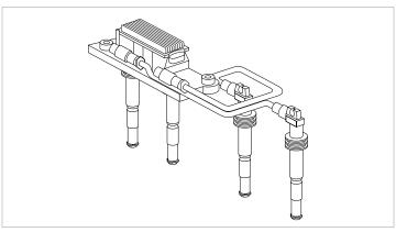
Ignition coils are mounted on the spark plugs for cylinders 2, 4 and 6. For example, for: Mercedes-Benz M104.
