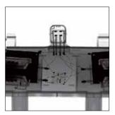
Copy: Wires running in every which way, distorted contact fields in the high-voltage connection, crooked coil bodies and boards: premature failure of the ignition coil is only a matter of time.
