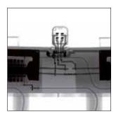
**Original:** Exactly placed and welded bus bars and components fixed straight into the housing in the original BERU part – a sign of quality and durability.
