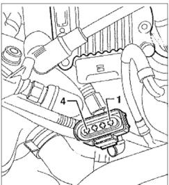
Switch off the ignition. Remove four pole plug from the ignition coil. Switch on the ignition. A voltage of at least 11.5 V must be present between contacts 1 and 4 of the removed plug. Switch off the ignition.
