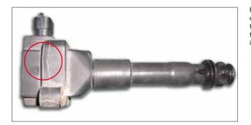
Formation of longitudinal cracks on coil body due to incorrect and excessive tightening torque of 15 Nm instead of the correct 6 Nm.
