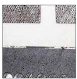
Copy: Separation between primary and secondary coil bodies due to unoptimized material pairings. This can result in leakage currents and disruptive discharge at the primary coil and thus lead to failure of the ignition coil.
