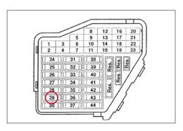
Testing the double spark ignition coil taking the ZSE 003 for VW / Audi as an example: The fuse must be OK (in this case: no. 29).
