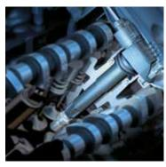
Plug shaft ignition coils are mounted deep in the engine compartment and must withstand extreme thermal loads
