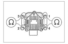
Measure secondary resistances of the ignition coils with ohmmeter at the high-voltage output. Outputs cylinders 1+4 / outputs cylinders 2+3. At 20 degrees Celsius, the nominal resistance must be 4.0–6.0 k $\Omega$ . If the values are not reached, the ignition coil must be replaced.
