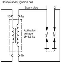
The voltage of 750 V is to low to allow an activation spark to arise.
