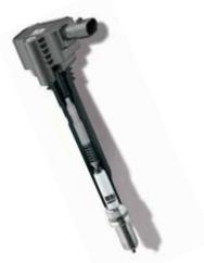
Space-saving and highly efficient BERU ignition system: double platinum spark plug with Plug-Top ignition coil. The internal pressure spring 'bowl' connector on the new double platinum spark plug prevents insulator flashovers.
