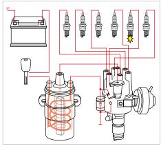
Triggering by contact breaker. In this case the voltage is centrally generated by an ignition coil and is mechanically distributed by an ignition distributor to the individual spark plugs. This kind of voltage distribution is no longer used in modern motor management systems.
